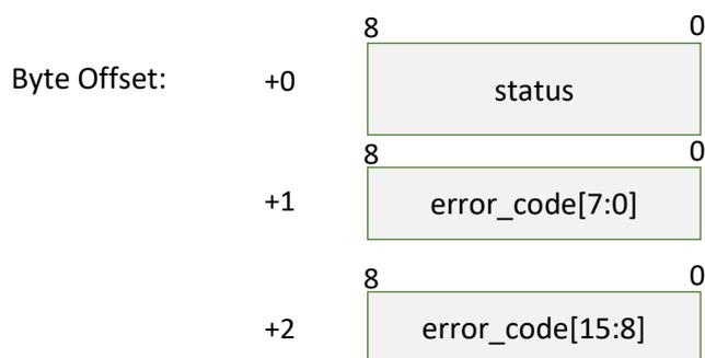
Figure 4-21 Format of a Device Health Data Response Packet
