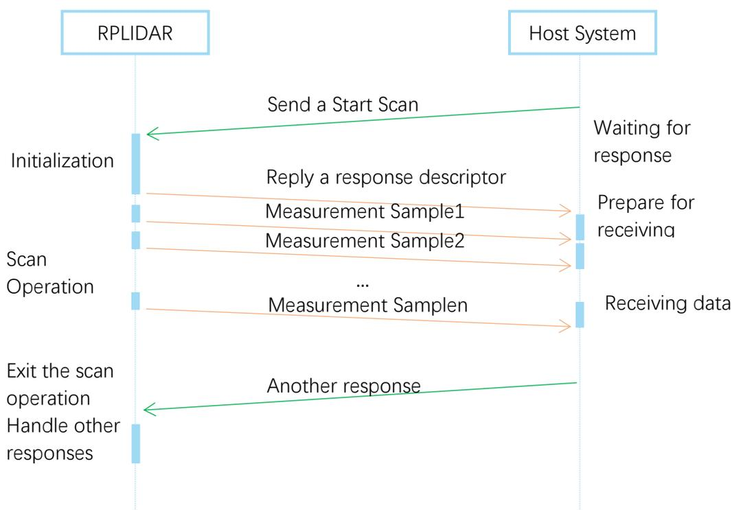
Figure 2-2 RPLIDAR Single Request - Multiple Response Mode
