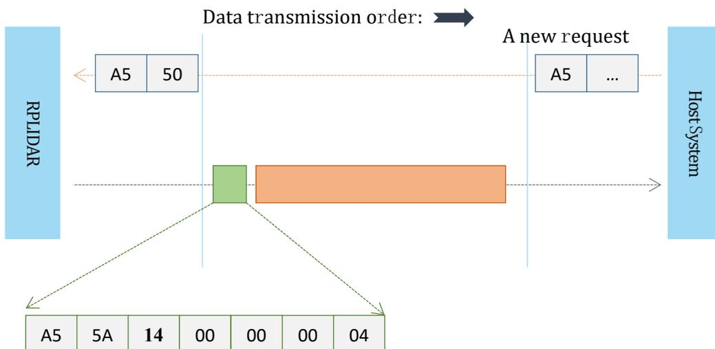
Figure 4-20 The Timing Sequence of a GET\_INFO Request
