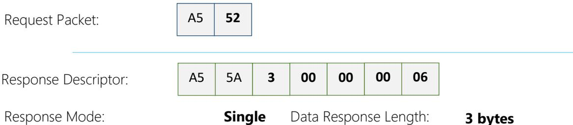
A host system can send the GET\_HEALTH request to query RPLIDAR's health state. If the RPLIDAR has entered the Protection Stop state caused by hardware failure, the related error code of the failure will be sent out.
