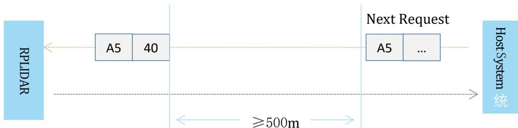
Figure 4-3 The Timing Sequence of a RESET Request
