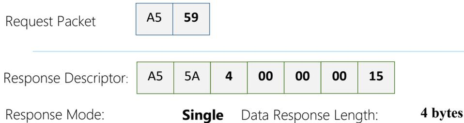
By sending this request, the host system can get the single measurement duration in standard scan mode and express scan mode respectively and calculate the current rotating speed of RPLIDAR accurately.
