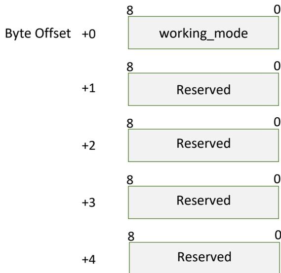
Figure 4-11 Format of a RPLIDAR Express Scan Data Request Packet
