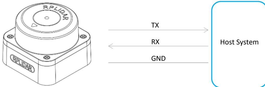
Figure 1-1 The Communication Between RPLIDAR and Host System
