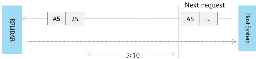
Figure 4-2 The Timing Sequence of a STOP Request
